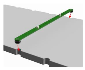
To position this 2-pin bar on such a couch, gently push the bar with its two indexing elements into a set of couch cut-outs. The bar itself should now be flat on the surface of the couch. Always make sure that the bar is well positioned on the couch before indexing the other hardware to the 2-pin bar.
