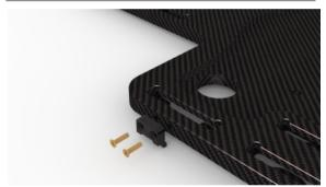
Mount the Loxon<sup>™</sup> blocks to the side of the base plate using the plastic countersunk M5 x 20 screws and a screwdriver.
