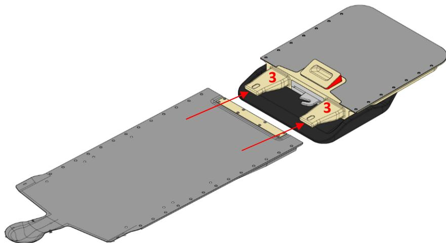
3. Slide the extension towards the base. By sliding the extension towards the base, the latch plate will turn into the locked position. The release handle – which is connected with the locking pin – will fall down into the locking position.
