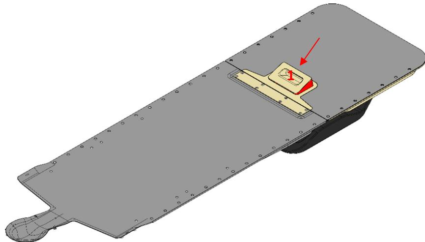
2. Grab the extension slide the extension outwards - in longitudinal direction – away from the couch base part.
