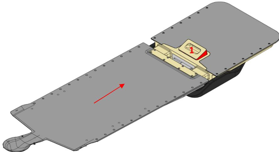
4. When the handle surface is flush with the top surface of the couch (the red unlocked sign is not visible), and when there is a small seam of +/- 1 mm between the couch base and the extension, then the couch extension is correctly secured to the couch base.
