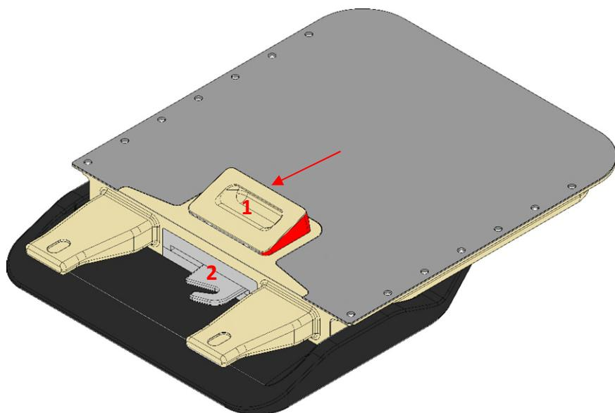
2. Grab the extension at the sides and hold the extension in front of the tabs and make sure the tabs (3) are positioned within the opposite cavities.
