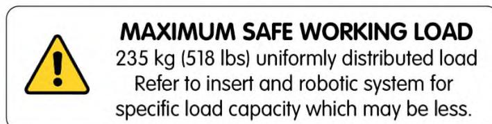
Do not exceed 235 kg (518 lbs) uniformly distributed load or maximum safe working load of the (entire!) couch top. The specific load rating of the extension or robotic system may be less. In that case, refer to their specific load capacity information.
