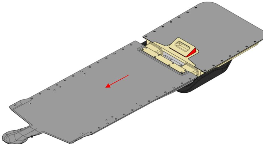
3. When reaching the stop (second safety mechanism), lift the extension slightly. **Make sure you hold the extension around the 'hand' pictogram stickers with two hands because the extension is heavier towards the bottom!** The weight of the extension is not evenly distributed.
