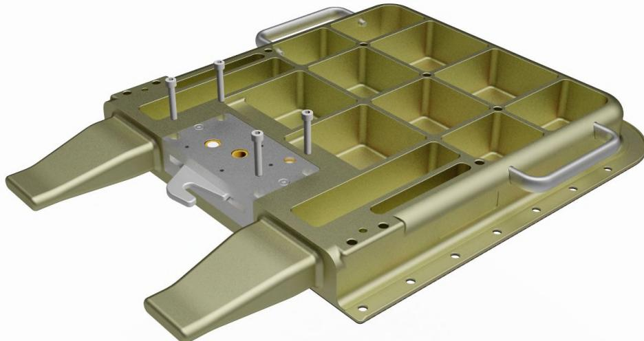
**Step 4:** the locking module can now be taken out. As the module is positioned with two dowel pins, you first have to move it out straight, before turning it out of the cavity as shown below. If it doesn't come out easily, you can (!) 'softly' knock or push on the release handle from the other side.
