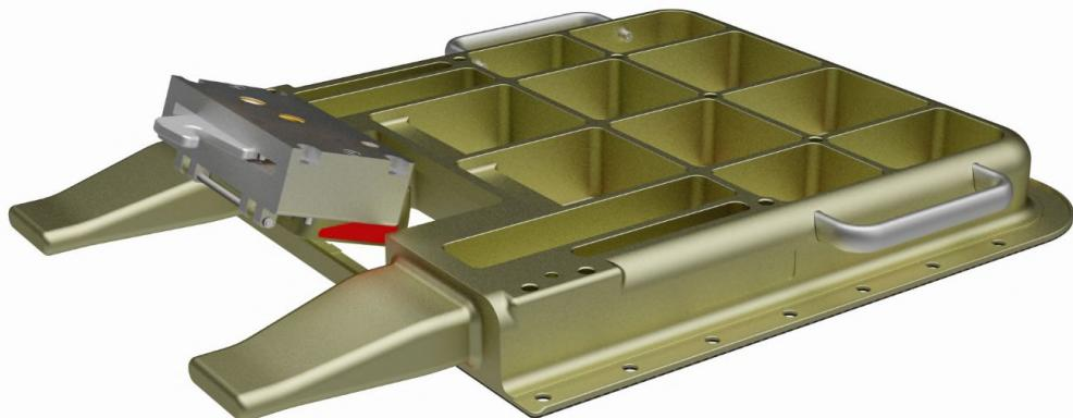
**Step 5:** the locking module is now disassembled.
