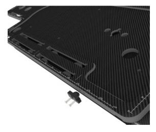
Mount the left side Loxon™ blocks to the left side of the base and the right side Loxon™ blocks to the right side of the base
