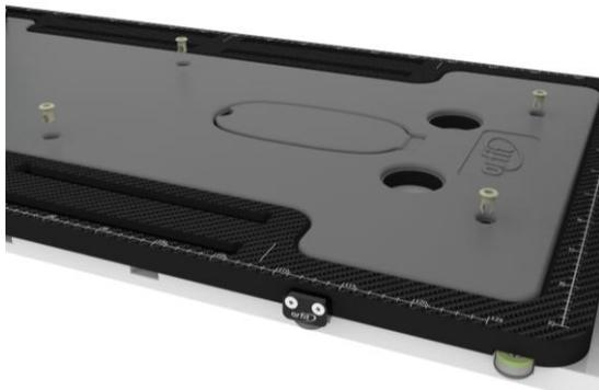
The 5° and 10° wedge cushions (38103 & 38102) can be indexed by inserting the widest part of the indexing knobs (38202) into the holes provided on the bottom side of the cushions.
